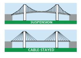
Figure 2 Suspension bridges including their cousin the cable-stayed bridge [13]
