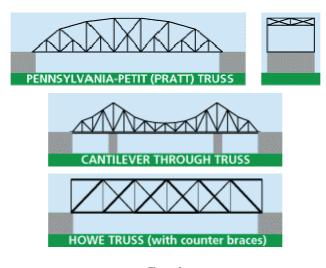
Figure 3 Bridges of Truss type [13]
