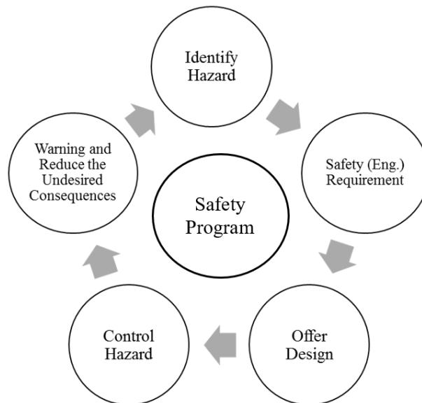
Figure 5: The Safety program.
