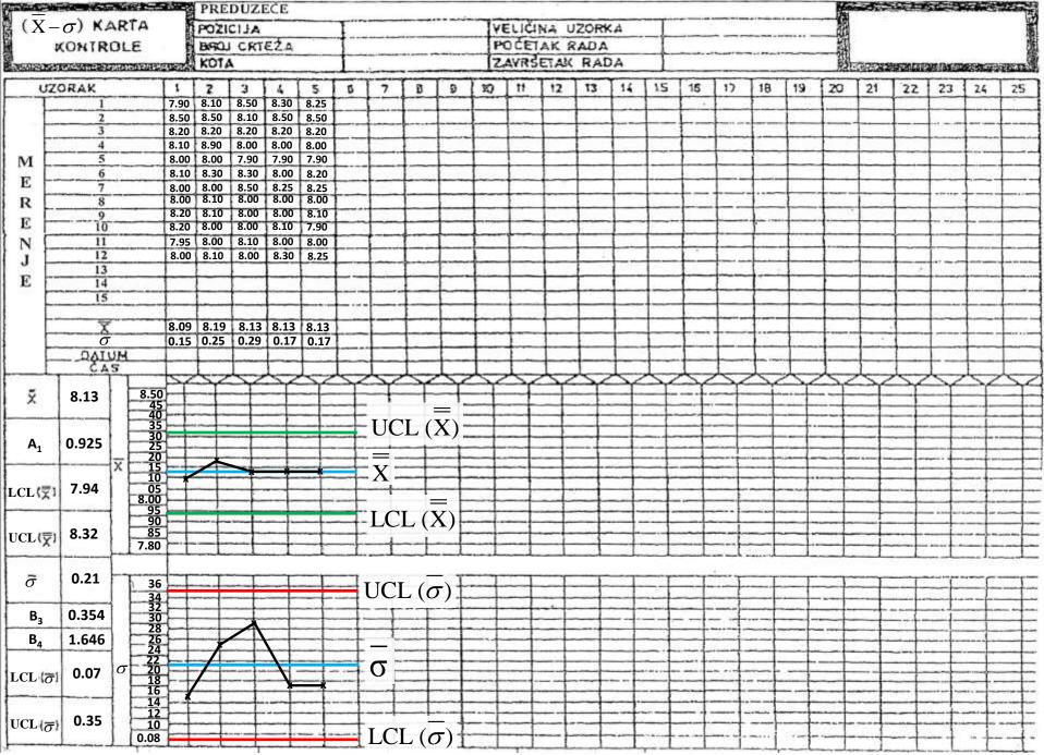
The process is under statistical control because all points fall within the UCL and LCL
